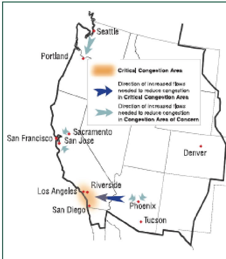
Figure ES-3. One Critical Congestion Area and Three Congestion Areas of Concern in the Western Interconnection
