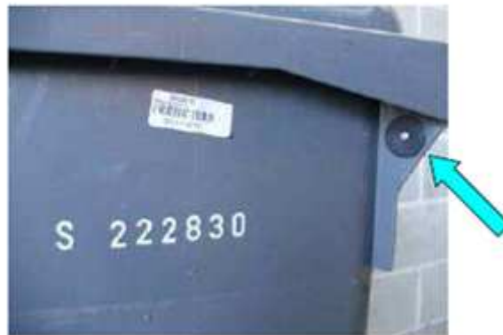
Figure B.4 A transponder for the identification of residual waste production.
