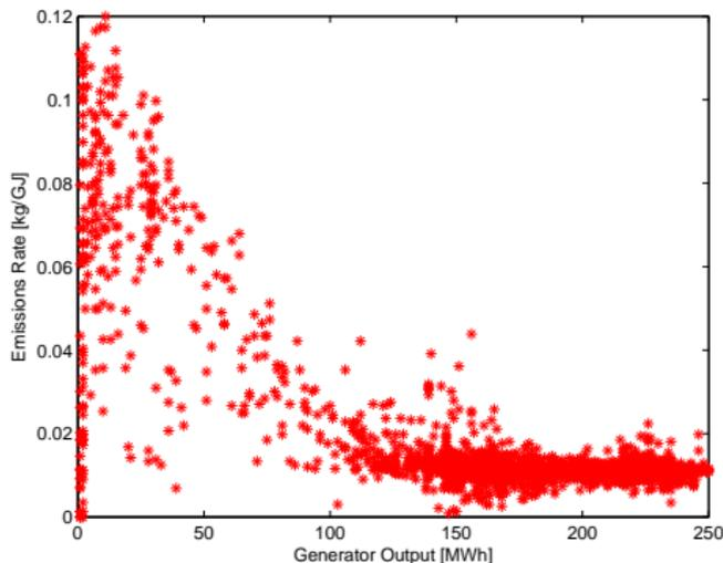
**Figure:** Measured NO<sub>x</sub> Rate of Wolf Hollow I CCGT *Source: US EPA CEMs*
