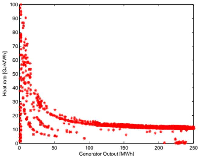
**Figure:** Measured Heat Rate of Wolf Hollow I CCGT *Source: US EPA CEMs*
