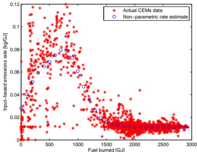
**Figure:** Non-parametric Estimate of NO<sub>x</sub> Rate of Wolf Hollow I CCGT *Source: US EPA CEMs*
