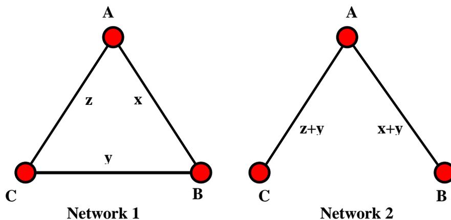
Consider for instance the traffic forecasts  $x$ ,  $y$  and  $z$  between nodes A and B, B and C, C and A respectively. If  $D_{ac}(z + y) + D_{ab}(x + y) < D_{ab}(x) + D_{bc}(y) + D_{ac}(z)$  where  $D_{ij}(\cdot)$  stands for the total cost function for traffic between  $i$  and  $j$ , it is worth to constraint all the flows between B and C to transit through node A. The solution will be minimal like Network 2 instead of the dense Network 1. The drastic solution is to never build line CB.
